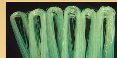
WLS fibers collect light produced in HEP hadronic calorimeters. They absorb blue and re-emit green so that as much light reaches PMTs.
