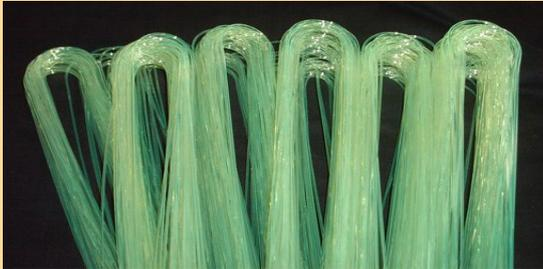
CMS Hadronic EndCap calorimeter is made of scintillator tiles with WLS fibers embedded. These fibers collect light produced in tiles. They absorb blue from scintillator and re-emit green so that as much light reaches PMTs.
